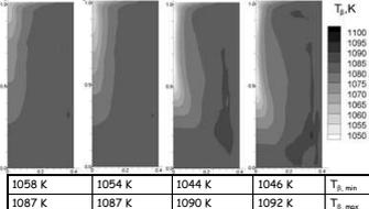
For microstructural control during heat treat, a narrow range of  $T_{\beta}$  is desired. Low power, buoyancy driven cases (2 on left) show much lower band of  $T_{\beta}$  than high power, electromagnetically driven cases (2 on right).
