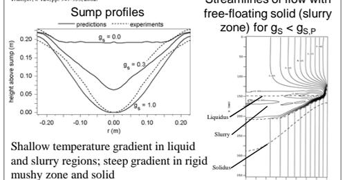
Shallow temperature gradient in liquid and slurry regions; steep gradient in rigid mushy zone and solid
