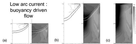
(a) Weak clockwise flow driven by thermal and solutal buoyancy forces is not strong enough to penetrate and break up stratification in liquid region. Because the flow is weaker than high power case, the overall final segregation levels (c) are much lower.
