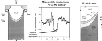
Direct Chill Casting, used to produce most of world's wrought aluminum, frequently exhibits severe negative centerline segregation. The numerical model examined role of free-floating, equiaxed grains on segregation patterns. Predictions indicated a significant decrease in centerline composition because of accumulation of Cu-depleted solid grains at bottom of sump.
