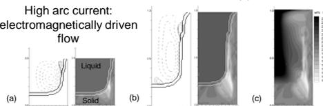
(a) Strong counterclockwise flow driven by electromagnetic forces stirs liquid region and removes Fe-rich, Al-depleted liquid from mushy zone during filling. (b) Once full, the current is turned off and flow is controlled by buoyancy. The liquid pool becomes stratified, leading to much higher segregation near centerline of final ingot (c).
