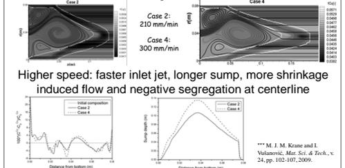
Higher speed: faster inlet jet, longer sump, more shrinkage induced flow and negative segregation at centerline
