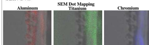
Figure 4. SEM Dot Mapping images display how the oxide layer of the 2000°F sample forms in separate layers, aluminum forming the first layer, followed by titanium, and outside layer of chromium.
