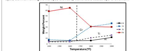
Figure 5. Displays the average elemental composition in weight percent in the oxide layer of four elements for the temperature range of 1400°F to 2000°F. Samples to the left of dashed line are a combination of matrix and oxide layer due to the spot size being large relative to oxide thickness.
