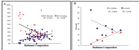
Figure 1. Plots of statistical analysis that were performed on the provided heat chemistry data. Plot A was generated from the complete data set of heats. Plot B was generated from master heats that contained similar compositions in all elements besides hafnium.
