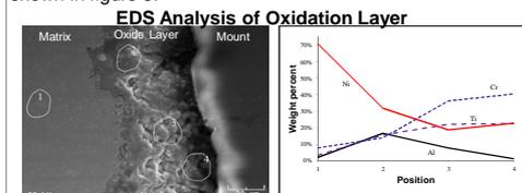
Figure 2. Secondary Electron SEM image showing oxide layer that resulted from exposure to 2000°F for 1 hr.
