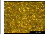
Sample exhibited a non-banded structure with ferrite and pearlite bands running parallel to the rolling direction. This particular sample contained 0.83 wt.% Mn.
