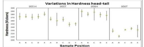
Microhardness testing throughout the thicknesses showed a clear variation in hardness both within and between samples
