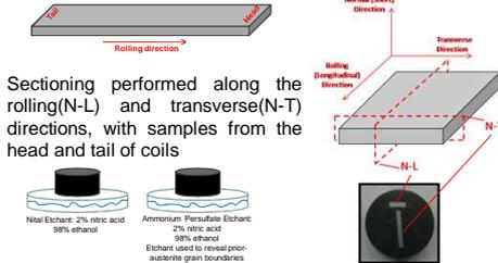
Metallography performed on all samples to evaluate phase fraction (Image J software), ASTM grain size, and for inspection of defects in the microstructure
