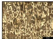
Coil #1 exhibited a banded structure with ferrite and pearlite bands running parallel to the rolling direction. This particular sample contained 0.83 wt.% Mn and had a large ASTM grain size of 10, which correlates to small grains. Pearlite area fraction was 6-15 times the ferrite area fraction.
