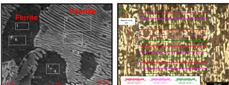
EDS (electron dispersive spectroscopy) performed in conjunction with the SEM to obtain compositions of Mn across the different phases (ferrite, ferrite+cementite)
