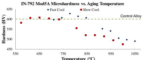
IN-792 Mod5A Fast Cooled (37°C/min) and aged from 710-1050°C for 8 hrs
