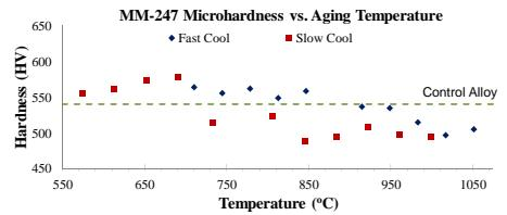
MM-247 Fast Cooled (37°C/min) and aged from 710-1050°C for 8 hrs
